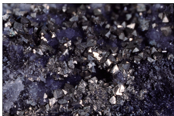
【Figure 8】 Jinguashi octahedral pyrite (with visible triangular crystal plane) is generally produced in environment of higher temperature
